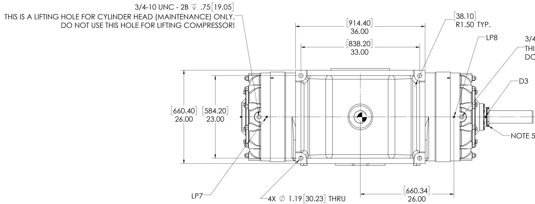
$3/4-10 \text{ UNC} - 2B \ \sqrt{\phantom{0}} .75[19.05]$ THIS IS A LIFTING HOLE FOR CYLINDER HEAD (MAINTENANCE) ONLY.
